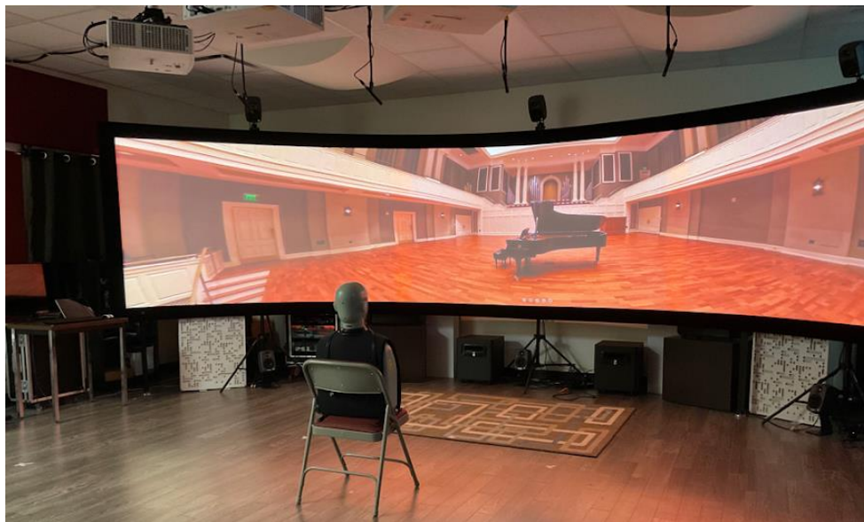
Figure 1. Piano recording in McAfee Concert Hall, Belmont University, using three microphone arrays (top); visual reproduction of the recording via a 250-degree wraparound screen, with 24 loudspeakers for 3D immersive audio reproduction in the RIT immersive experience laboratory (bottom).
